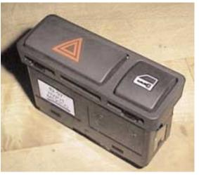
The opened door can be re-locked when closed by manually locking or pushing the central button twice. This allows the locks of the remaining doors to be re-synchronized again.
